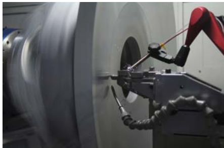
Ultra-precision treatment of the 60 cm mirror
